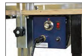
Built In Transformer
